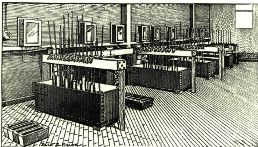
Figure 1.1: Drawing of Hall's original electrolytic cells.
