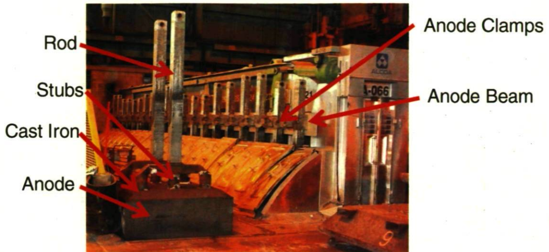
Figure 2.4: Baked carbon anode assembly.
