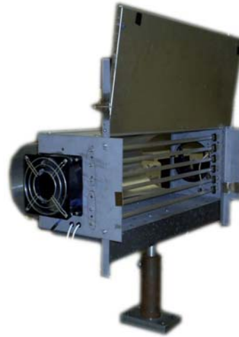
Heating lamp 6 infrared tubes 1.2 kW each Shutter-solenoid configuration Minimum pulse duration: 300 ms
