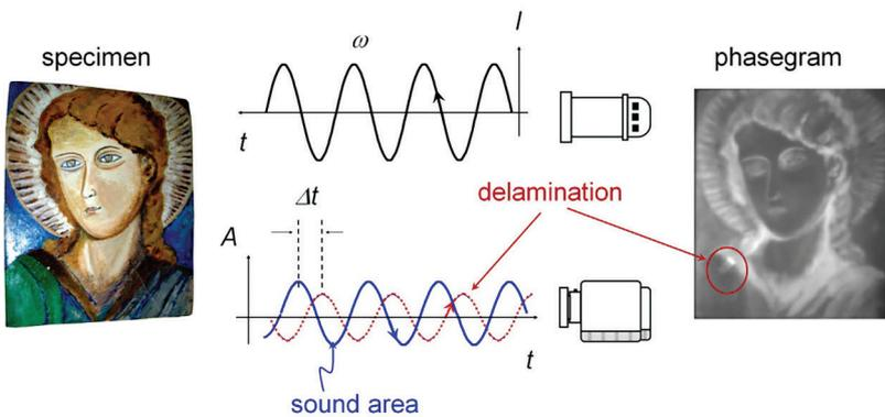
Figure 3. Modulated thermography stimulation following a sine pattern. Top: signal injected into the specimen; bottom: collected return signal exhibiting a shift in time between defective and non-defective zones due to the propagation into the specimen. Phasegram image shown on the right (for the specimen shown on left)
