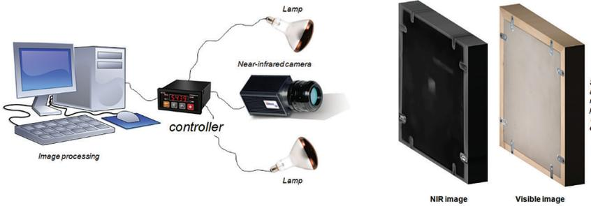
Figure 1. NIR set-up with 0.9-1.7 μm camera
