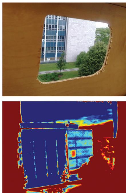
Figure 8. Visible photograph of Vachon building on Université Laval's campus (top) as seen through a hole in a veneer panel from a nearby building. Bottom: MT phasegram image recorded after cyclic solar heating over six days
