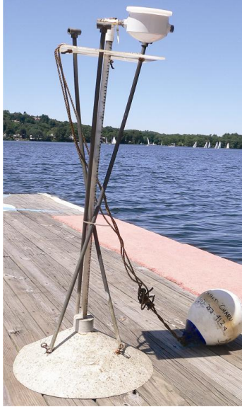
Figure 1-4: Image of a bubble trap on a dock at UML. The funnel at bottom collects gas bubbles into the PVC cylinder, and the buoyancy of the gas column allows the pressure sensor at top to estimate the collected volume. The traps were suspended about 1 m below the water surface by the buoy. Courtesy of Charuleka Varadharajan.
