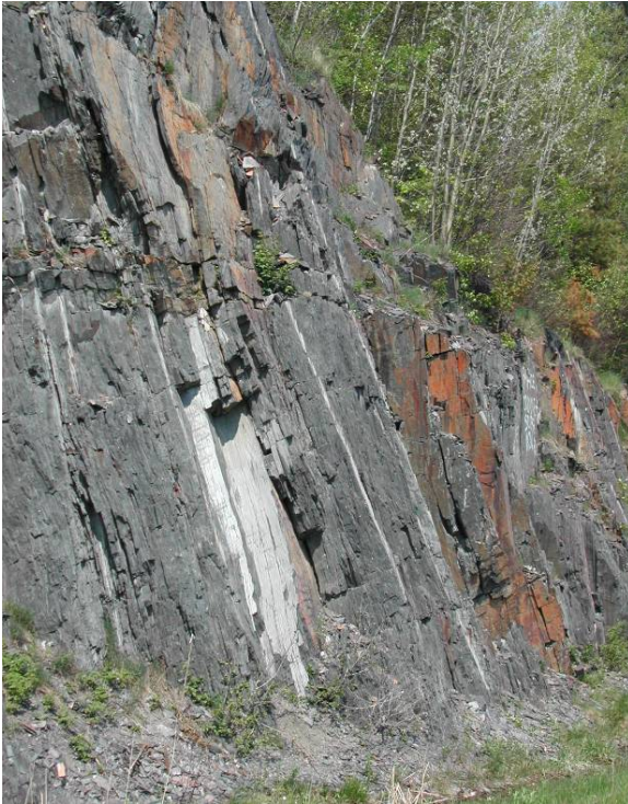
Figure 15: Schistose rock in eastern part of the exposure (Fleurimont rock slope, May 24, 2007)
