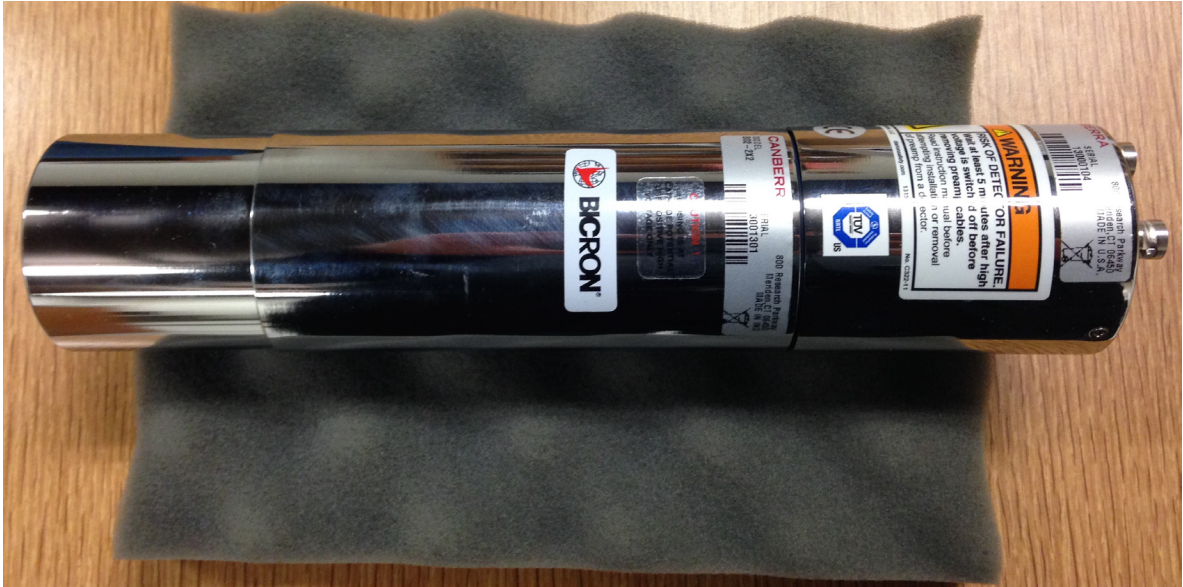
Figure 12. Canberra model 802 NaI(Tl) scintillation detector with PMT.
