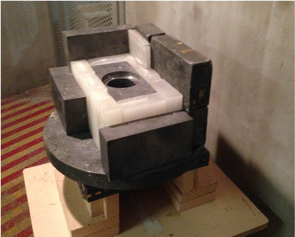
Figure 2. Shielding for the neutron source.
