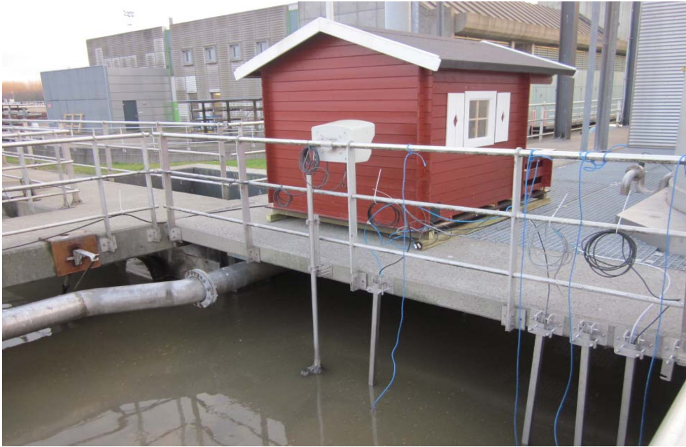
Figure 2 – The monEAU monitoring station installed at the inlet of the primary clarifier at the Lynette wastewater treatment plant in Denmark
