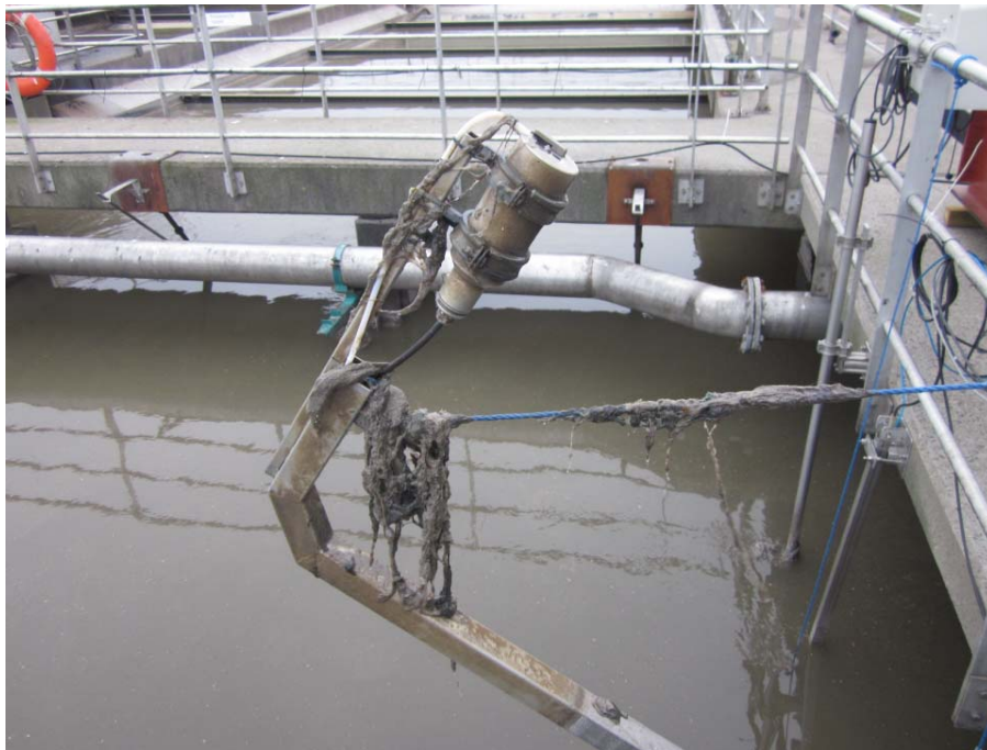
Figure 6 – The case study turbidity sensor – Sensor fouling problems
