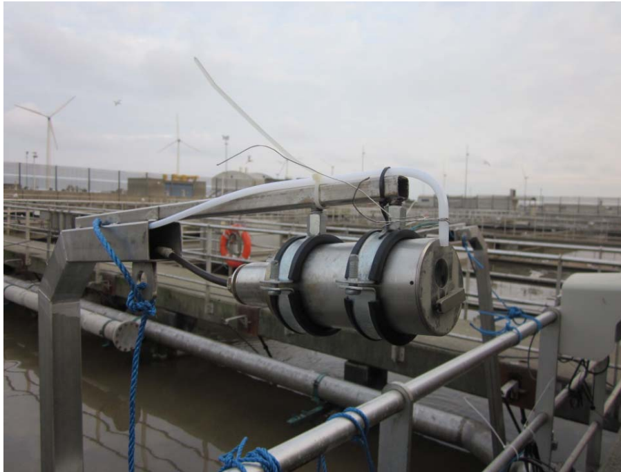
Figure 5 – The case study turbidity sensor installed at the primary clarifier of the Lynette wastewater treatment plant in Denmark
