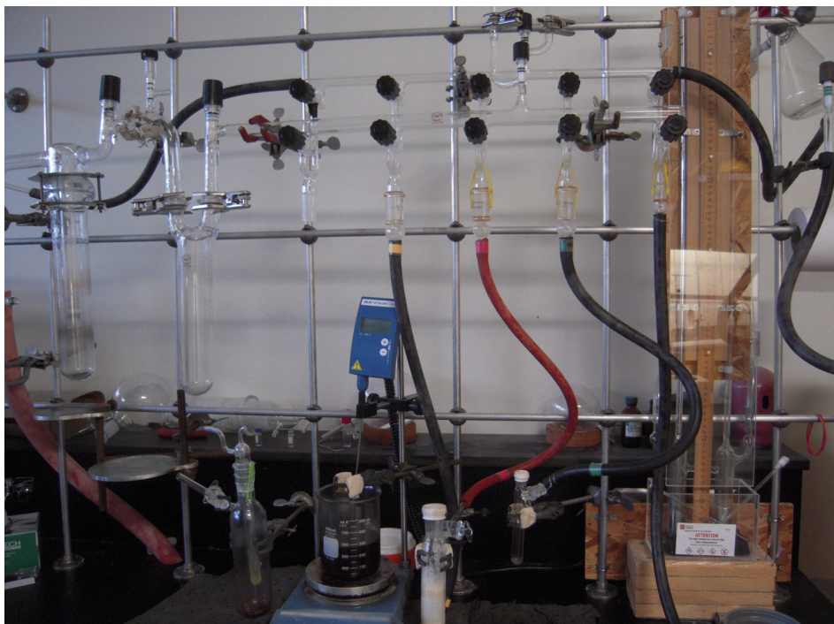
Figure 3.1: Double manifold Schlenk line and Schlenk tubes used in inert atmosphere chemistry.
