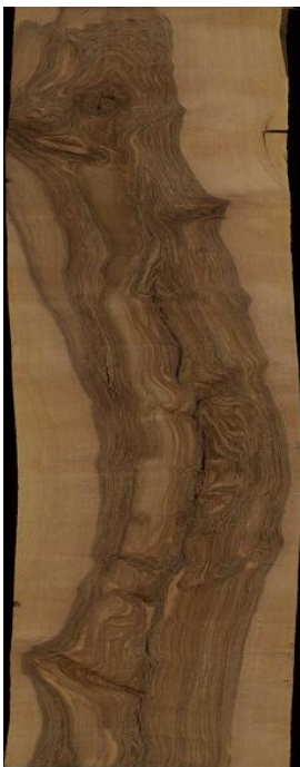
Figure 3.9 Example of a difference in color homogeneity between sapwood and discolored wood regions. While sapwood is homogeneous in color, discolored wood presents different shades and creates a marble effect to the eye.
