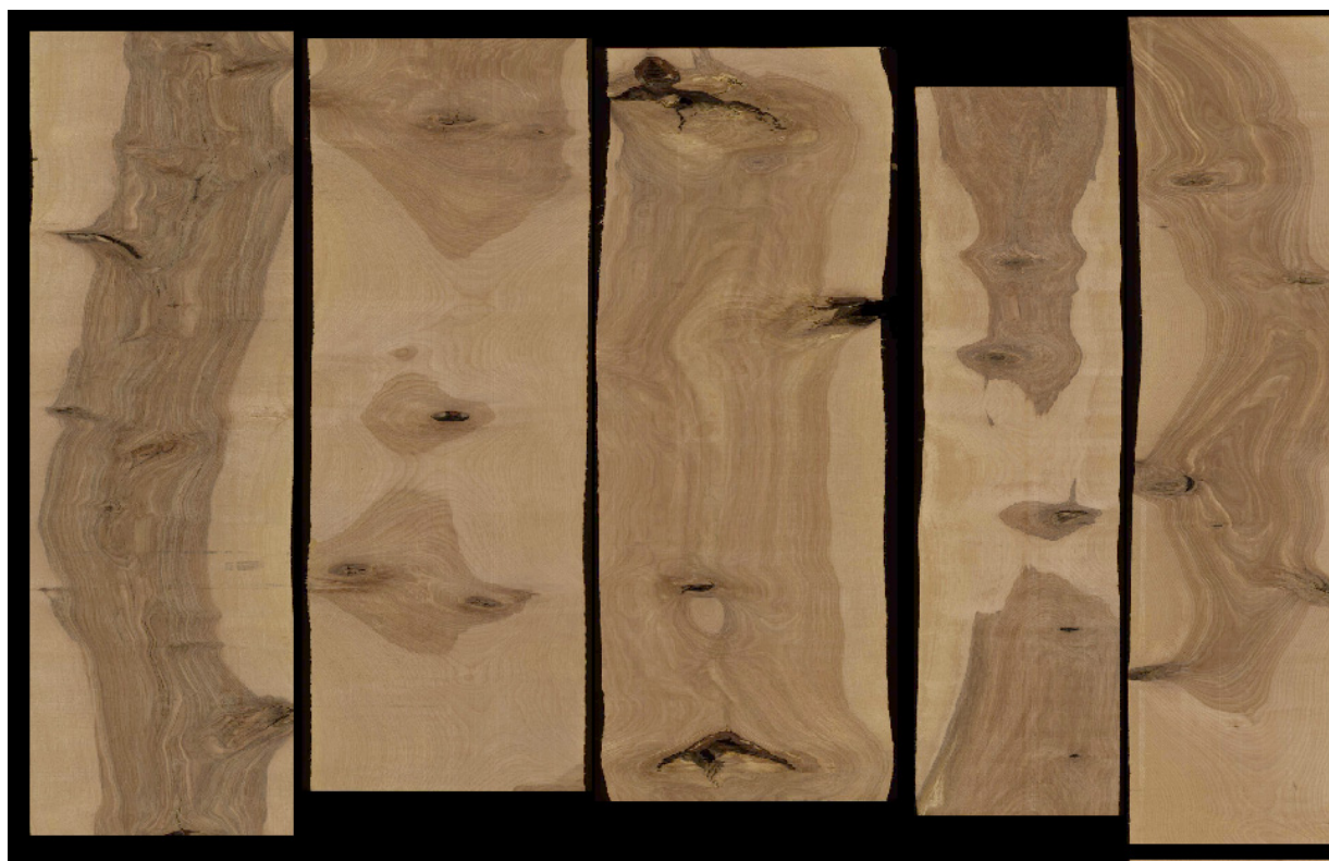
Figure 3.7 Digital images of boards showing the relationships between discolored wood and character marks where most of the time, knots and wounds are found in discolored wood areas.
