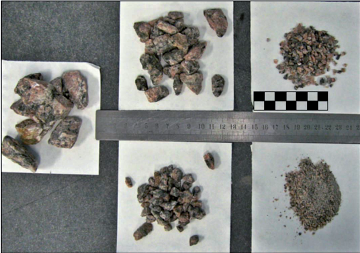
Figure 4-7- Angular granite grains with different particle sizes used in preparation of the triaxial specimens
