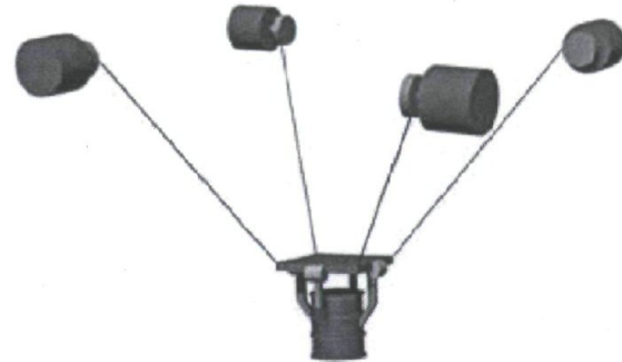
(d) A spatial cable-driven mechanism handling potentially hazardous material [7]
