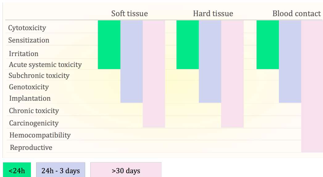
Figure 2.7. Common testing requirements for corrosion resistant materials (CRMs) based on ISO 10993 and ASTM 1983 standards. Depending on the implant site, CRMs are required to be assessed based on the listed test. Blood contact CRMs need to meet the requirements for hemacompatibility and reproductive-related assessments. Adapted form [25].
