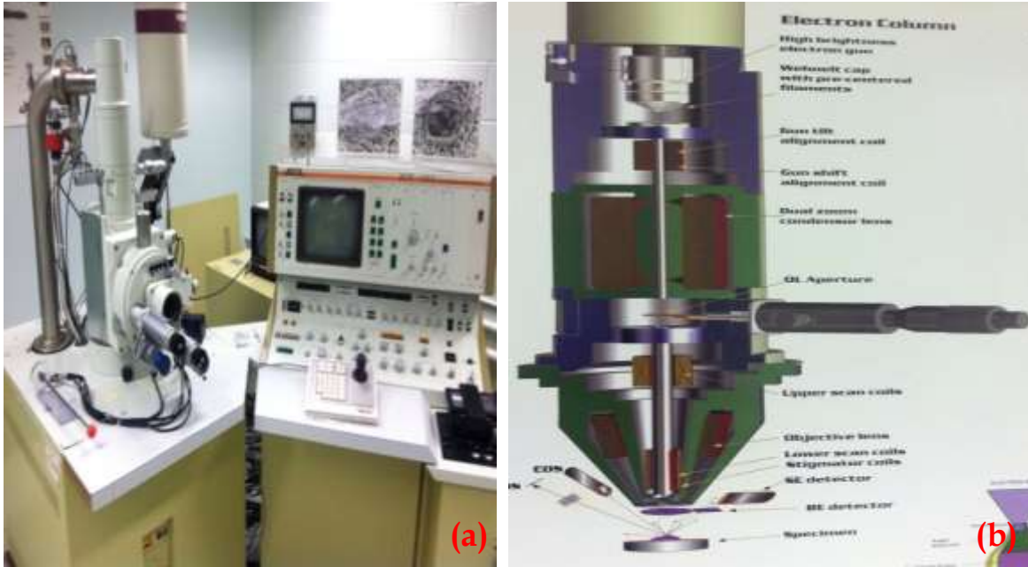
Figure 3.6: JEOL SEM – JSM 840A, (a) Set – up, (b) working procedure
