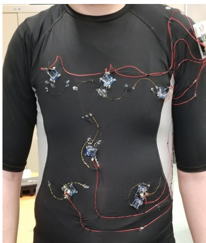
Figure 2.21 – The smart T-shirt with six breathing sensors
