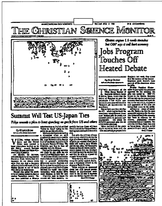
Figure 6.1 The layout after edge detection. The block boundaries are fairly well defined, but the image is full of spurious artifacts — noise, boundary breaks and other discontinuities.
