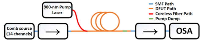
Fig. 8. Setup used to measure the gain and NF of fiber A and B.
