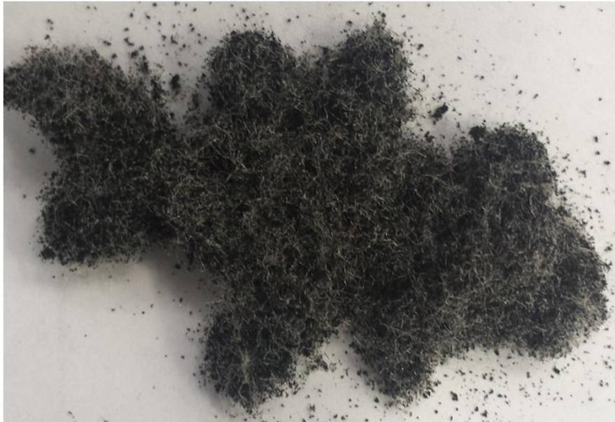
Figure 2.2. General view of the polyester recycled tire fibers (RTF) mixed with ground tire rubber (GTR) as received.
