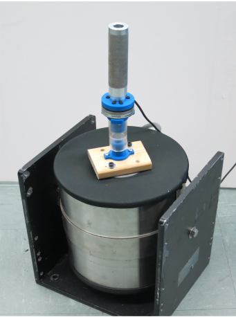
FIGURE 1.23 – Presentation of the setup used to generate vibrations with a shaker during a hose insertion.
