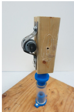
FIGURE 1.21 – Presentation of the setup used to generate vibrations with an unbalanced mass and a motor during a hose insertion.
