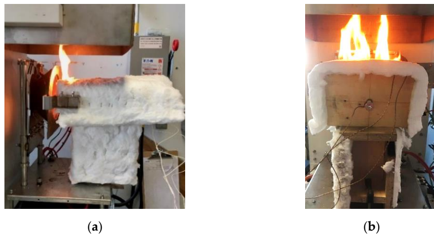
Figure 2. Fire test using conical radiant heater at 50 \text{ kW/m}^2 : (a) Experimental setup with the fastener head exposed (side view); (b) Experimental setup with the fastener tip exposed (back view).
