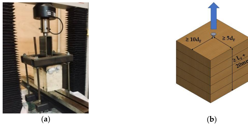
Figure 3. Pull-through STS test: (a) Experimental setup for the pull-through test; (b) Location of STS across glulam surface.
