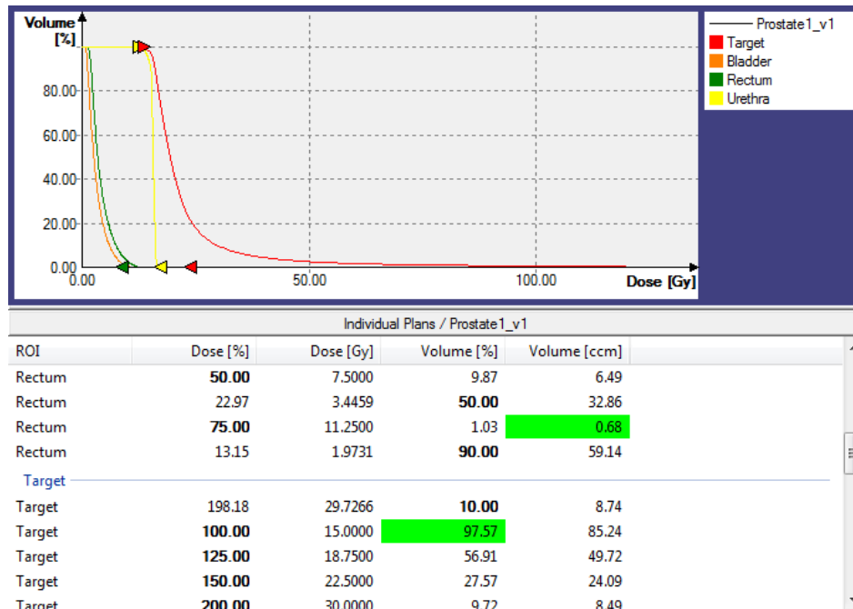
FIGURE 0.11 – DVH results and dosimetric parameter results (the recommended ones for evaluations are highlighted) of an optimal treatment plan for prostate cancer in Oncentra Brachy (top: cumulative DVHs, bottom: dosimetric parameters).
