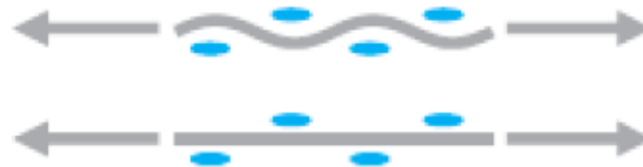
Figure 2-9: Straightening of the yarns in case of uniaxial tension (14)
