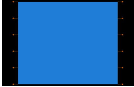
Figure 6-9: Application of the loads on the shell element for a simple extension test
