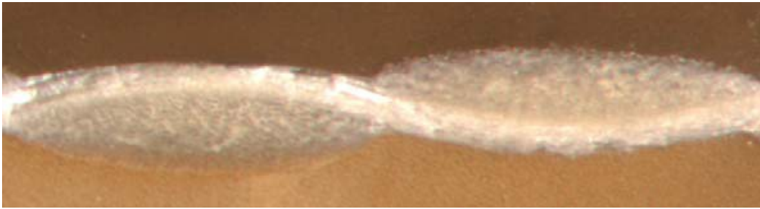
Figure 3-9: Cross-sectional micro-image of a plain weave fabric made of Kevlar fibers (2)
