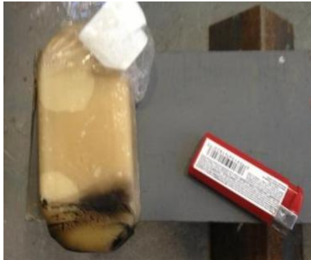
Figure 3-7: The adhesive mounting method used to fix the accelerometers on the beam surface.
