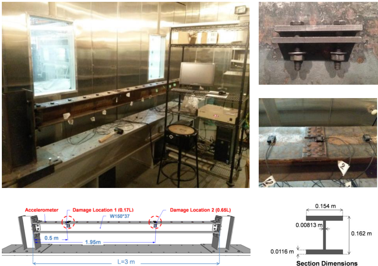
Figure 3-1: A schematic representation of the beam showing the beam in its fully bolted configuration state.
