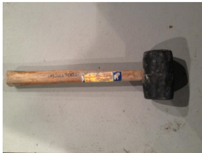
Figure 3-5: Impact hammer used to induce dynamic random excitations on the beam.
