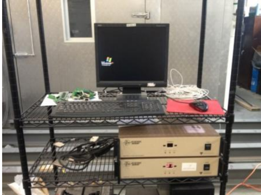
Figure 3-8: StrainSmart® data acquisition system, model 6100.
