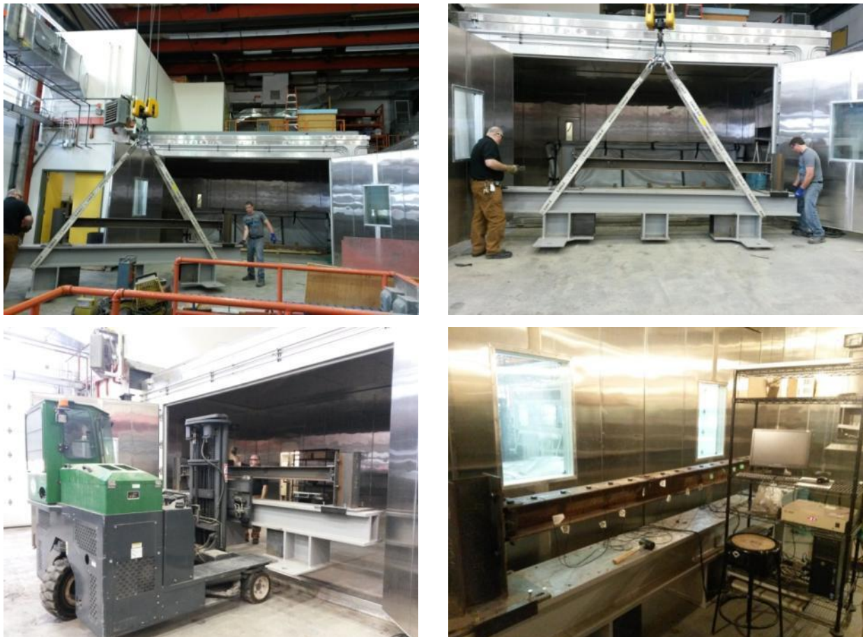
Figure 3-10: Step-by-step moving process of the beam in the climate-controlled room.
