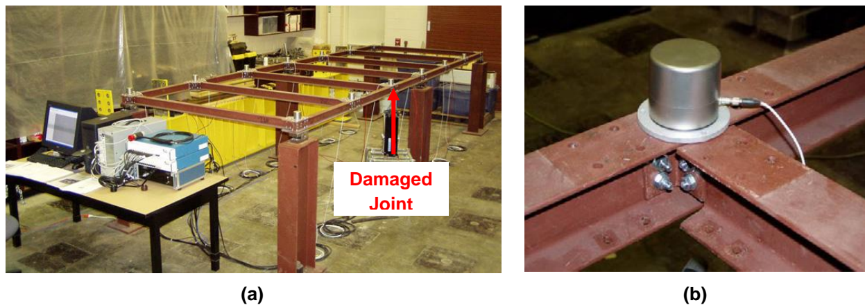
Figure 2-7: The steel grid model in the laboratory, a) instrumentation of the model, b) loss of stiffness by removing cover plate from the top and bottom of the girder (Catbas et al. 2007).
