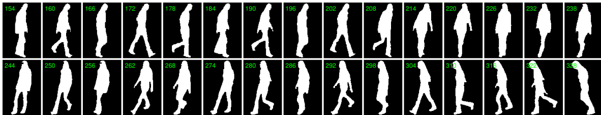
Figure 2.4 – Results of background subtraction and morphological filtering for 30 frames of a video sequence. Only the relevant portion of the binary frames are shown.
