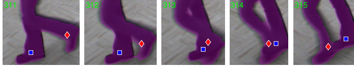
Figure 2.11 – Examples of foot location and tracking with occlusion. The silhouette is overlaid in pink in the frames, and the foot positions are represented by a blue square and a red diamond. In frames 311 and 315, the feet are not in occlusion since the legs can be separated by analyzing the legs region of the silhouette. Frame 312 to 314 correspond to occlusion frames since there is no background gaps between the legs (frame 313), or the height of the background paths is not long enough (frames 312 and 314).
