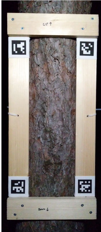
Figure 2.1: This figure shows a sample of zoomed red pine images from our dataset. The wooden frame used to surround every bark surface in our dataset is displayed with its four fiducial markers.
