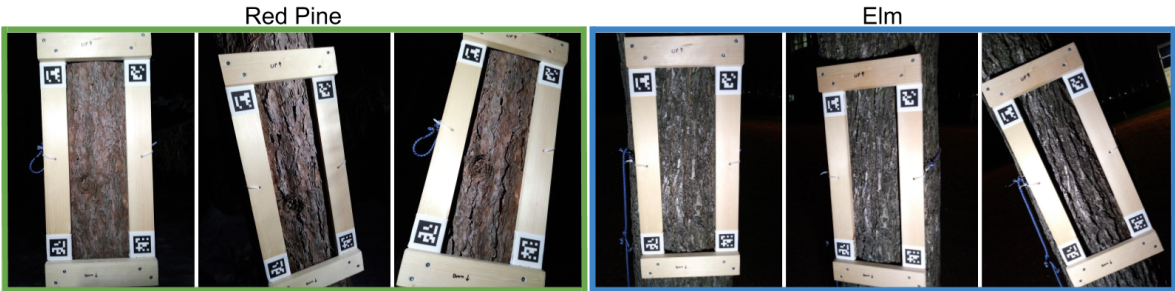
Figure 2.2: Images from our database of Red Pine (RP) and Elm (EL). For each species, we can see three images of the same bark surface, but for different illuminations and camera angles. In each image, there are four fiduciary markers on a custom-made wooden frame, used for pixel-wise registration.
