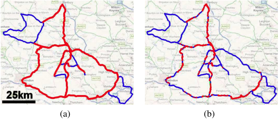
Figure 1.1: Figure taken from Cummins and Newman (2009). This figure shows a 1,000 kilometers trajectory with loop closure in red. The (a) panel provides the ground truth, and the (b) panel provides the detected loop closures by the Fab-Map 2.0 algorithm. They correctly detected 2,189 loop closures and predicted six false positives. This gave them a 99.8% precision at 5.7% recall. In the original caption, they mentioned that the long section with no loop closure detected is a highway at dusk.
