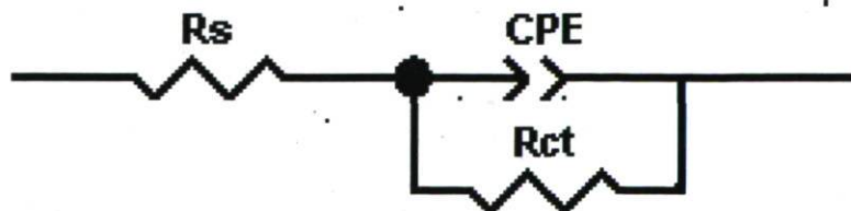
Figure 7.3 – Equivalent circuit proposed for fitting the experimental data of electrochemical impedance measurements of oxygen evolution reaction on lead-silver alloy anodes.
