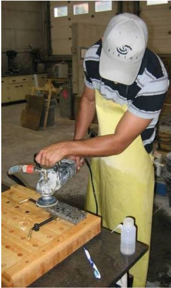
Figure A1.3: Polishing operations used for the preparation of plane polished slabs from which small concrete specimens were cut to perform micro-scratch testing. The method consists in wet polishing with diamond-coated rubber disks of different grit sizes.
