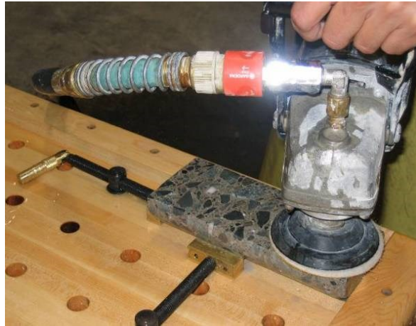
Figure A1.3: Polishing operations used for the preparation of plane polished slabs from which small concrete specimens were cut to perform micro-scratch testing. The method consists in wet polishing with diamond-coated rubber disks of different grit sizes.
