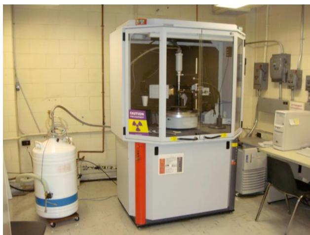
Figure 3-3: Bruker Apex II Diffractometer that is operated by our group.
