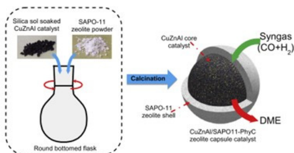
Figure 1.11- Preparation of CuZnAl@SAPO-11 catalyst by physical coating method (Reprinted with permission from [271]. Copyright 2015 Elsevier.).
