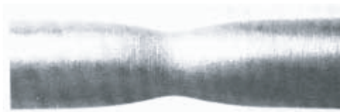
Figure 4.4: Cylindrical specimen necking under tension
