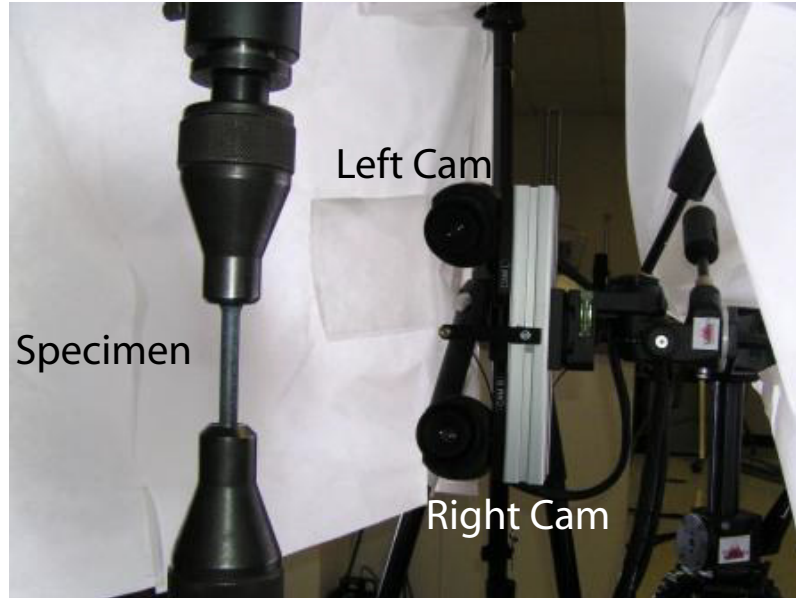
Figure 5.6: Back view of Aramis and the tensile test specimen.
