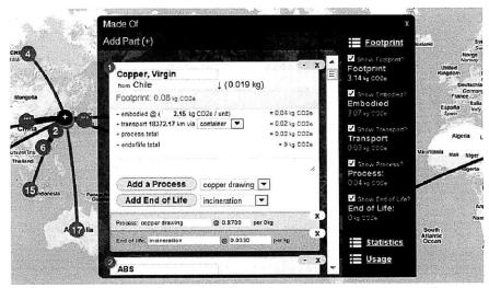
The 'Made of' dialog box acts as a Bill of Materials for each sourcemap: for every part, a user specifies the type of material, its provenance, weight, mode of transportation, processes and end-of-life strategy. The cumulative 'Receipt' is seen on the right.
