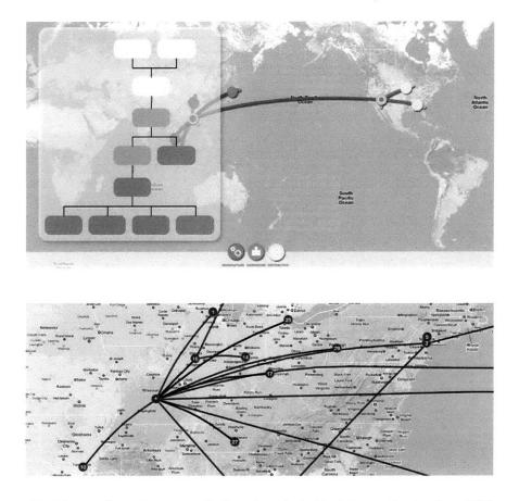
Prototypes of new Sourcemap features targeted at logistics professionals: a BOM is displayed as a tree diagram on a large touch-screen map (top); a drag-and-drop supply chain map supports multi-stop paths for individual parts (bottom)
