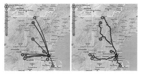
Stylized drawing of a supply chain (left) as compared with the actual routes taken (right). More realistic routing is being developed to accurately reflect distances, modes of transport and their relative environmental impacts.
