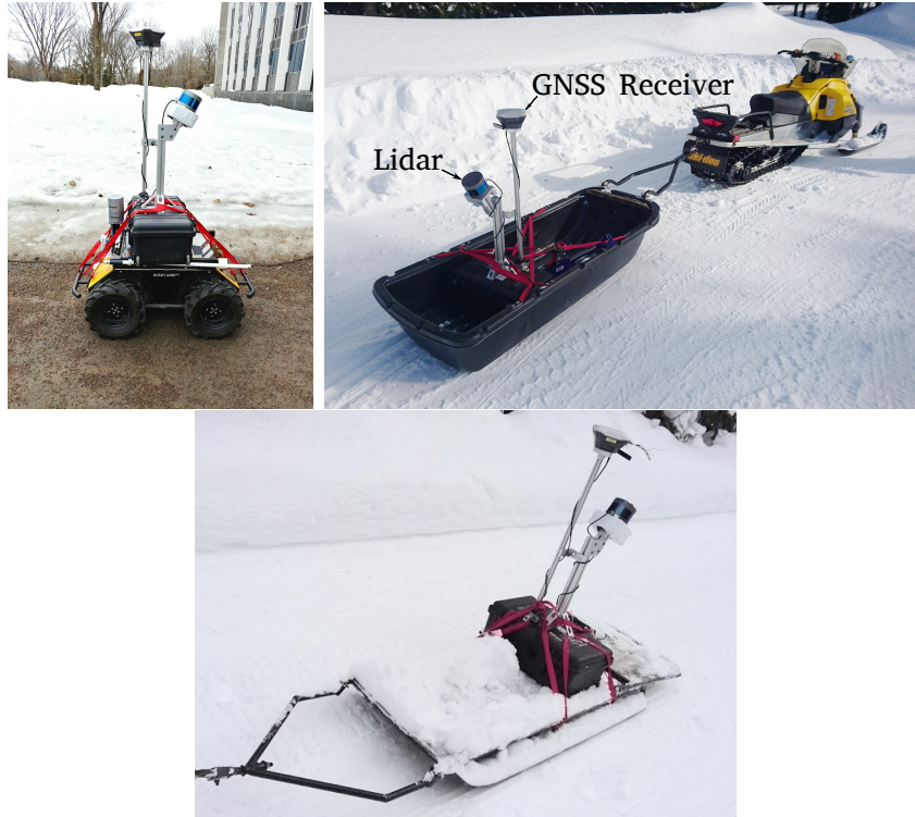
FIGURE 5.5 – Left : Rack mounted on a small robot for easy terrain (e.g., parking lot, sidewalks). Middle : Rack pulled by a snowmobile for maps on hardened snow. Right : As a last resort, the rack could be pulled by humans, which has proven to be useful on narrow/dense paths in the forest.
