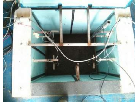
(b) Sensors support at the outlet of the Grandes-Piles F/AL.
