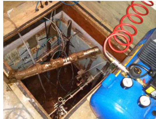
(a) Matter accumulation attached on a sensor's cable. (b) Matter accumulation on a sensor.
