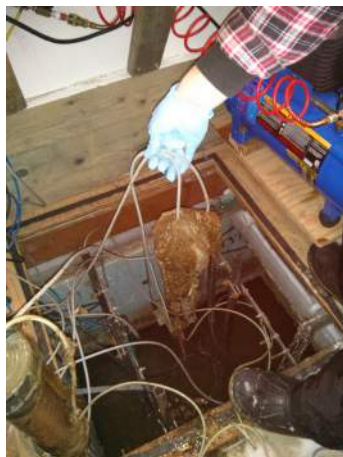
(a) Matter accumulation attached on a sensor's cable. (b) Matter accumulation on a sensor.
