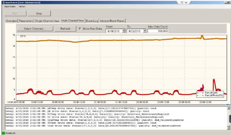
Figure 3.13: Influent temperature and pH time series on a graph on BaseStation software interface (Primodal, 2015a). Data collected at Grandes-Piles
