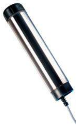
Figure 3.17: Hach LDO sensor used in the RSM30 stations.
