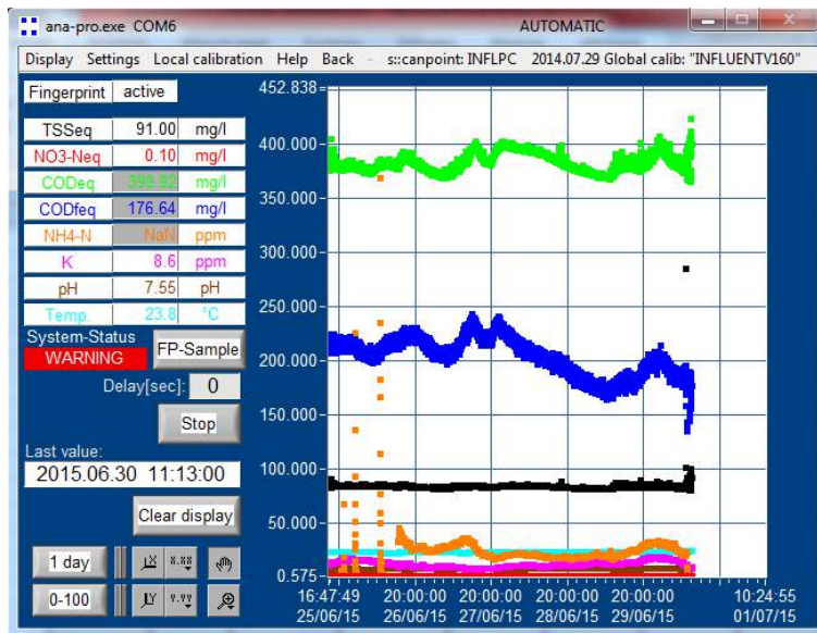
Figure 3.14: ana::pro software interface for two different s::can sensors (e.g. spectro::lyser and ammo::lyser) (s::can, 2006).
