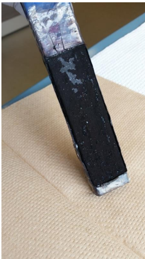
Figure 2.2. Lead-silver anode, showing manganese deposition.
