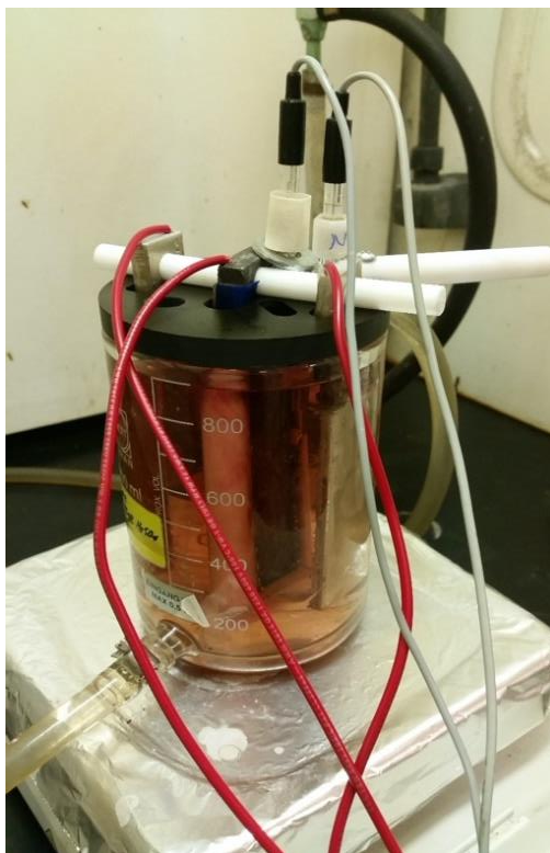
Figure 2.3. Cell of manganese removal system, using the galvanostatic technique.
