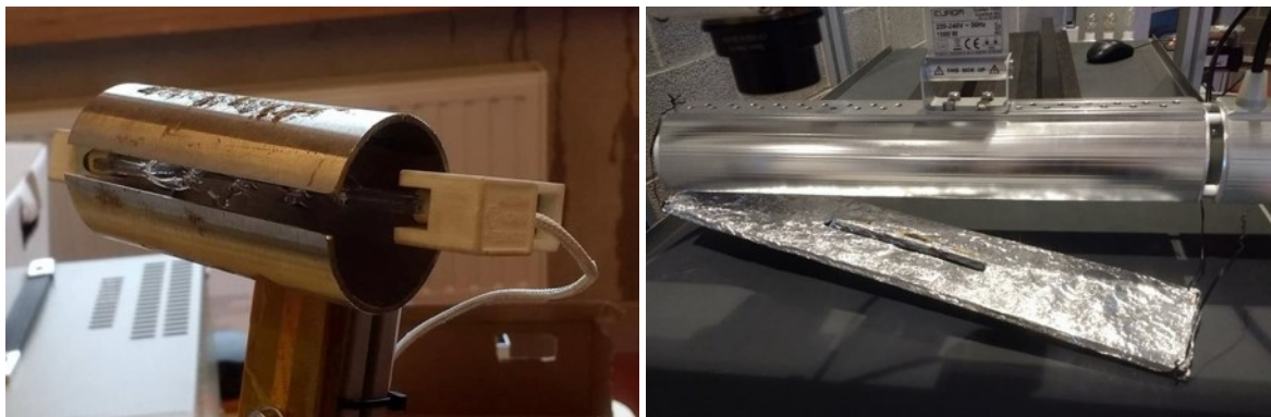
Figure 1. Two experimental set-ups are displayed as they are used in our lab: (Left) cylindrical reflector constructed to concentrate the radiation in a narrow line. This heater is used in dynamic measurements as a hand-held heater. Starting from a hollow tube a slit was milled with the desired width in order to create the reflector shape. (Right) empirical test-setup for Dynamic Line Scan Thermography on a conveyor belt. A wooden plate wrapped in aluminium foil was mounted underneath a patio heater. In the middle of the plate, a slit with desired width and length was cut in order to create the reflector shape. Both setups use a thin slot to minimise the heated region. Only the electromagnetic radiation passing through the slit will heat up the specimen to be inspected. Other rays will be blocked and thereby a large amount of energy is wasted.
