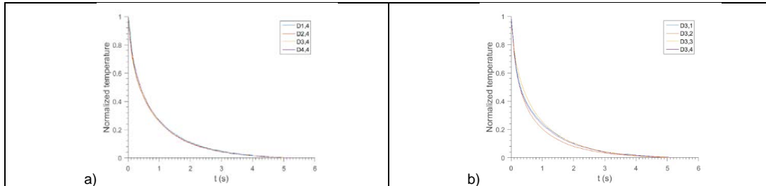
Fig. 9. Flying line scan active thermography: (a) thermal profiles: defects at the same depth and (b) defects not the same depth.
