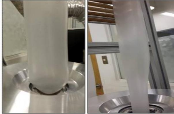
**Figure 2.4** Left: bubble cooled by the cooling ring. Right: bubble cooled by ambient air presenting the bottleneck phenomenon.
