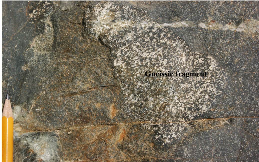
Figure 11- Photography of a decimetric gneissic fragment contained in a mineralized olivine-melanorite at the Outardes-4 South prospect.
