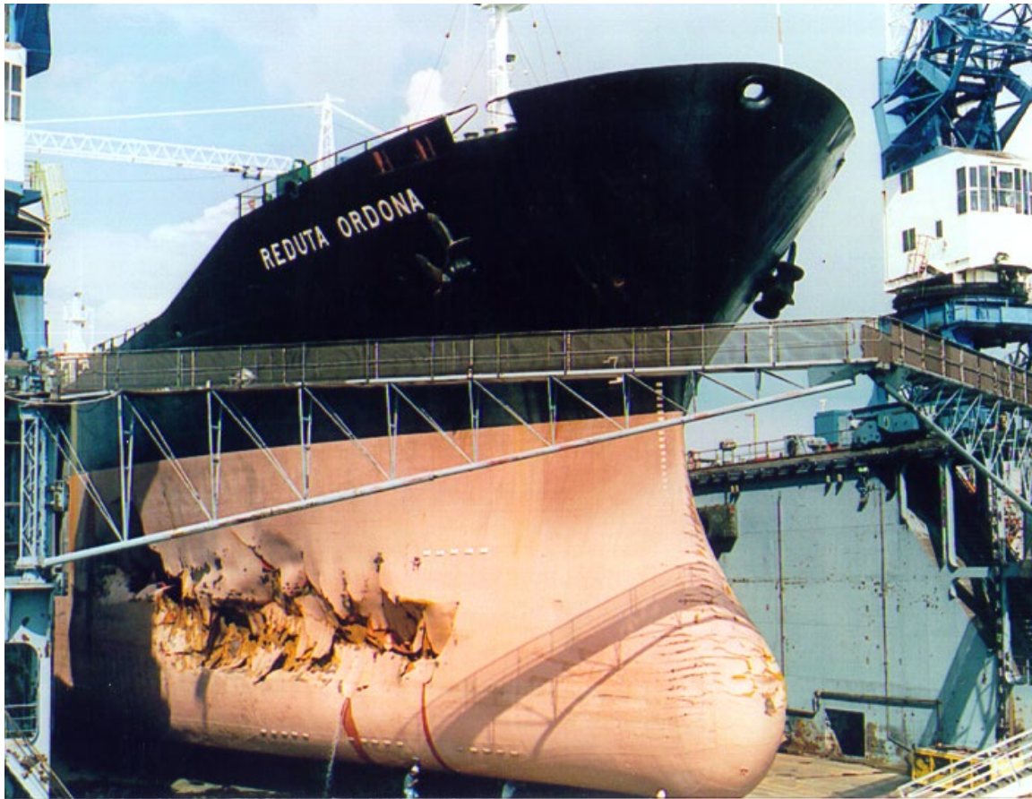
Figure 8 - The effects of the Reduta Ordona collision with a growler in Hudson Strait on its way from Poland to Churchill, Manitoba, July 21, 1996. Quebec City, MIL Davie shipyard.
