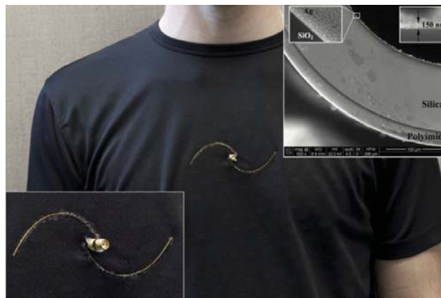
Figure 1. Prototype of the spiral antenna integrated into a cotton shirt, in the inset—SEM images of the multi-material fiber structure.
