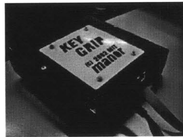
3.3.4 Box protecting A/D board
