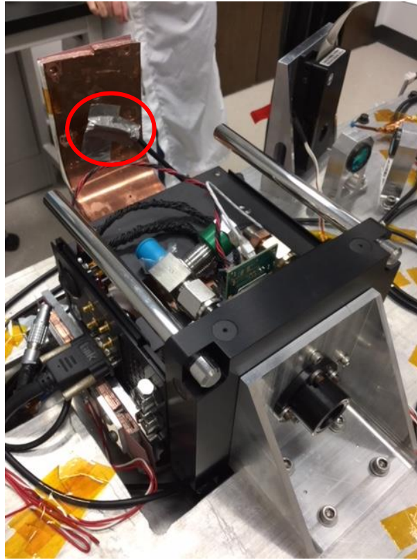
Figure 58: Thermocouple placement for the 128 Detector strap
