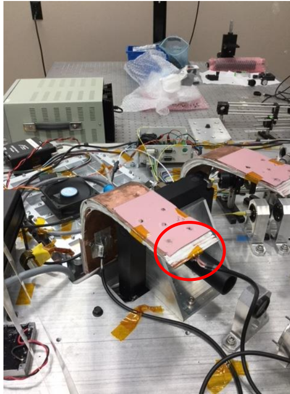
Figure 56: Thermocouple placement for the 512 Detector strap
