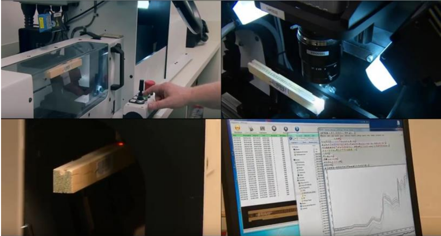
Figure 3.3 Automated system for near-infrared spectra collection from increment cores, developed by Centre de Recherche Industriel du Québec for Ministère des Forêts, de la Faune, et des Parcs du Québec, Canada. This system uses a motorized carriage (top left photo), a high resolution on-line camera (top right photo), and a 2-mm diameter near-infrared probe (bottom left photo) controlled by software (bottom right photo).
