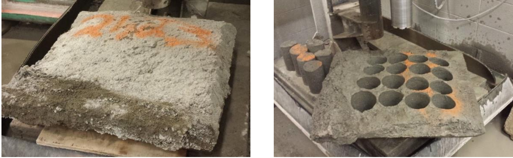
Fig. 6.4 Shotcrete test panel (left) and cored samples (right)
