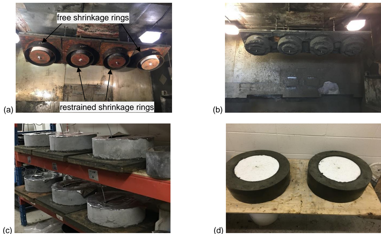
Fig. 6.3 Inclined overhead setup used to spray the shotcrete ring test specimens; (a) setup before spraying, (b) setup after spraying, (c) sealed instrumented restrained ring specimens, and (d) free ring specimens
