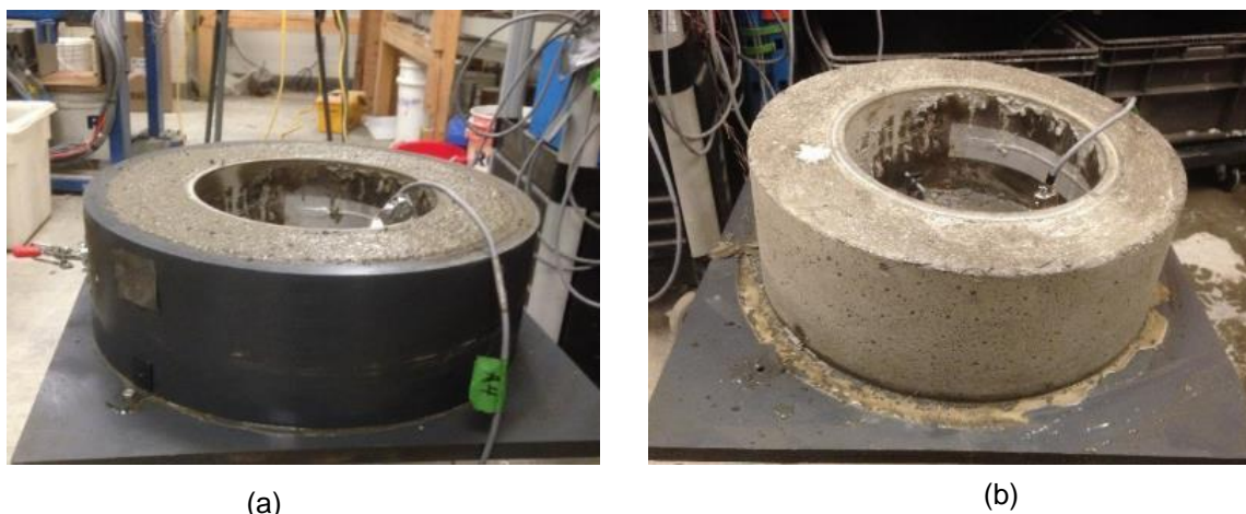
Fig. 2.7 Ring specimen with inner steel ring and outer PVC, immediately after gravity-casting; and b) after removal of the outer PVC form
