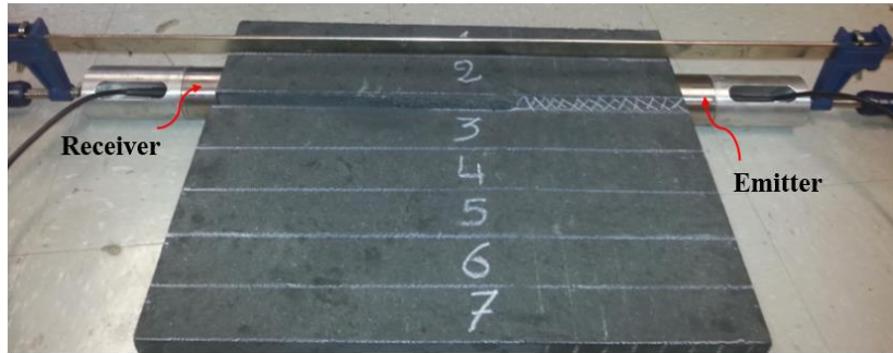
Figure A2-3 Acoustic data acquisition set-up through different corridors of an anode slice.
