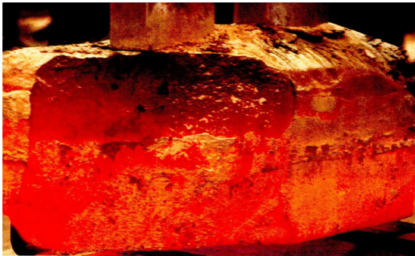
Figure 1-6 Cracked carbon anode due to the thermal shock in the electrolysis cell [50].
