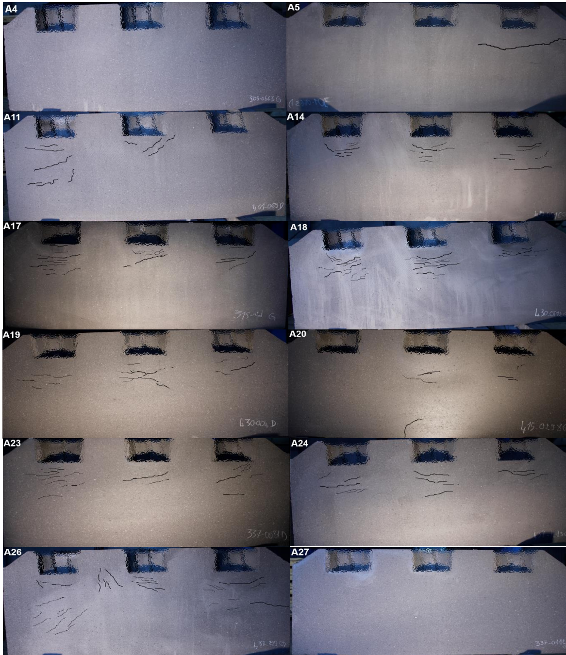
Figure 5-7 Images of cuts made on some tested baked anodes. The anode number is indicated in the top left corner of each image.
