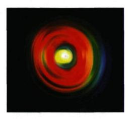
Figure 2-5: Beam pattern of a 7 mJ, 800 nm, 45 fs free propagating laser beam at far field (after filamentation).
