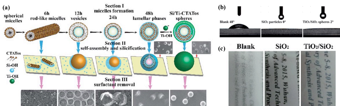
Figure 1.12: (a) The in situ synthesis mechanism of TiO 2 /SiO 2 nanospheres. (b) Contact angle of the blank substrate, substrate with SiO 2 particles, and substrate with TiO 2 /SiO 2 nanospheres. (c) The anti-fogging property of the samples. “ In situ growth of TiO 2 /SiO 2 nanospheres on glass substrates via solution impregnation for antifogging”, Liu, F.; Shen, J.; Zhou, W.; Zhang, S.; and Wan, L., RSC Adv. , Volume 7, Issue 26, 2017, Pages 15992-15996. Published by The Royal Society of Chemistry.
