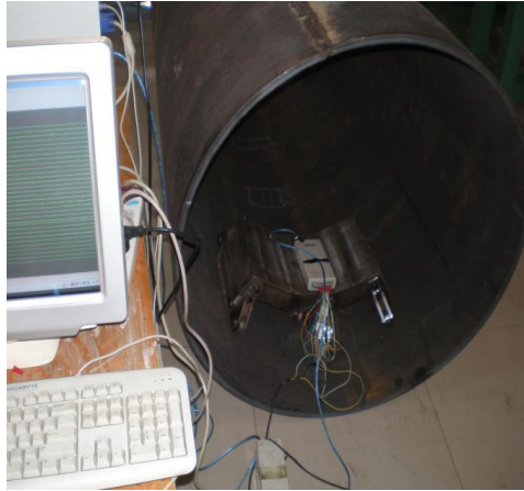
Fig.10 Experimental platform of circumferential MFL inspection
