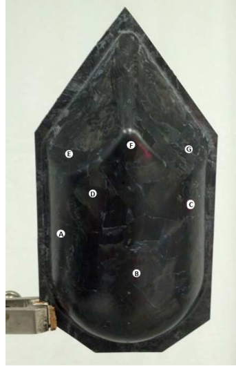
Figure 7. Tested points on the part's surface. Part's size is 8.4 \times 16.4 \text{ cm} in the real world.
