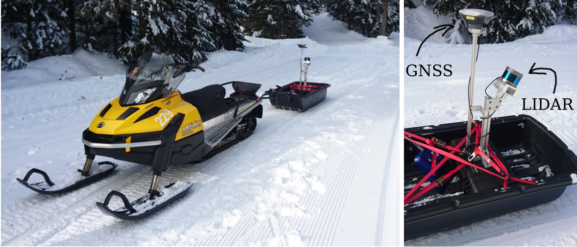
Figure 3.2 – The data acquisition platform mounted on a sleigh behind the snowmobile ( left ). This configuration limited transfer of engine vibrations to the sensors. Right : close-up of the GNSS receiver and the RS-16 lidar.
