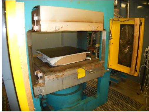
Figure 3-1 Dieffenbacher (862 mm by 862 mm) hot-press used to produce panels with homogeneous density.
